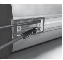
The sensor position is easily adjusted by undoing a set screw and using the cable to move the sensor to the desired position.
