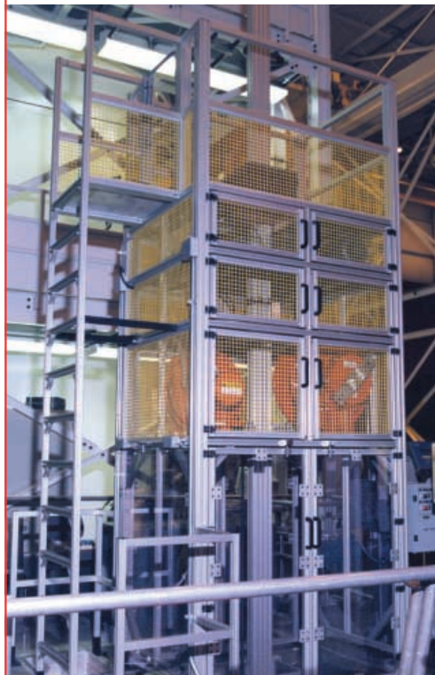
Support structure for drilling apparatus to clean spent fuel remains from space shuttle solid fuel rocket boosters
