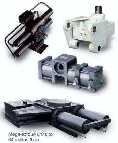
HRN Pressure Displacement Torque Series Bar (PSI) cm<sup>3</sup>/rad (in<sup>3</sup>/rad) Newton Meter (lb-in) 69 (1000) 2.12 (0.13) 1**0**S 10 (87) 3.61 (0.22) 20 (173) 15**S** 69 (1000) **20S** 69 (1000) 5.09 (0.31) 29 (260) **30S** 69 (1000) 10.82 (0.66) 59 (520) 100**S** 69 (1000) 23.55 (1.44) 123 (1089) 200S 69 (1000) 46.90 (2.86) 314 (2779) 400S 69 (1000) 92.31 (5.63) 539 (4770) 700S 69 (1000) 165.52 (10.1) 980 (8673)
